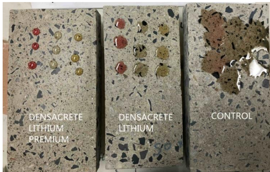
Figure 2. Oil beadings (engine oil, olive oil & heavy engine oil) at the start of test
