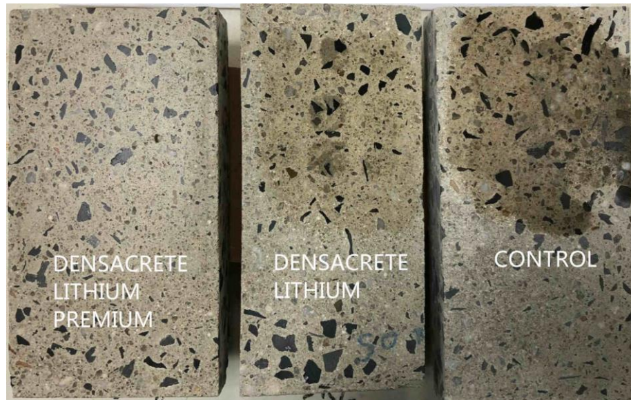
Figure 4. Oil stains (engine oil, olive oil & heavy engine oil) after 24 hours
