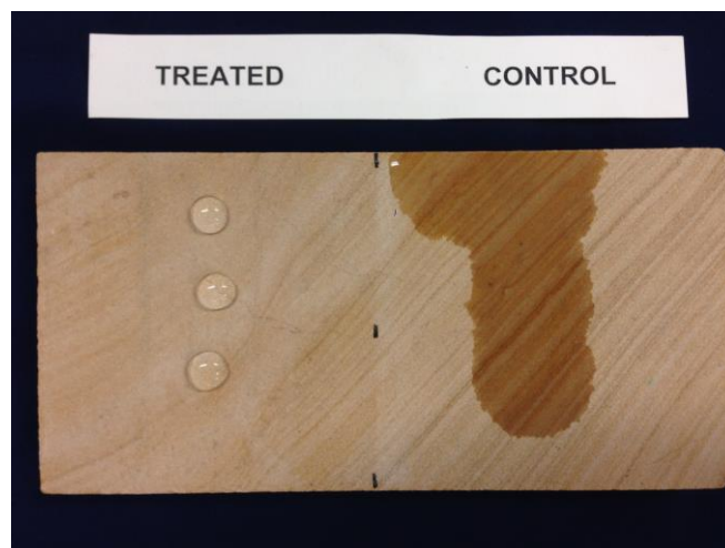
Figure 1. Surface Beading Achieved by Emulsion GPE50P
